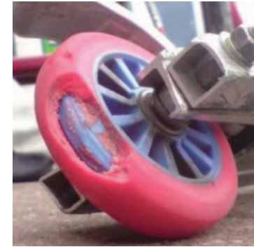
http://www.scooterresource.com Broken scooter wheel (sign of bad engineering design) due to poor material choice or poor loads assessment.
