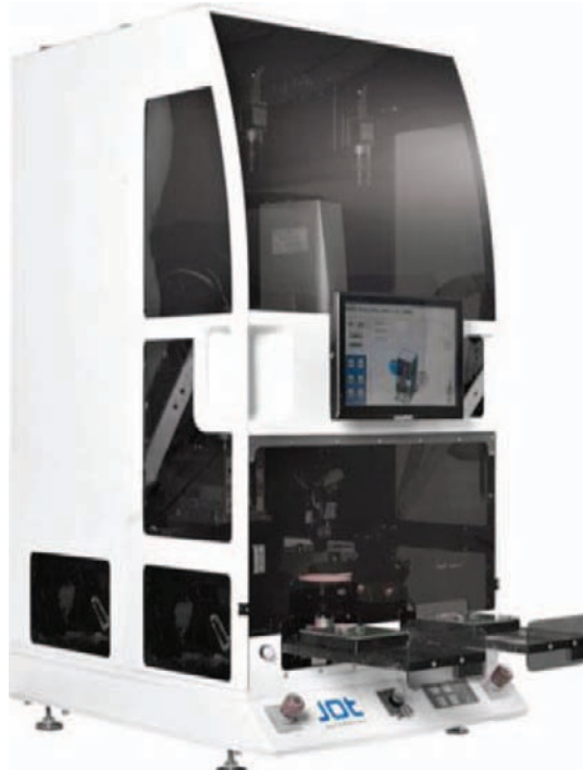
JOT V4 assembly cell and visual assembly quality control by Cognex camera
