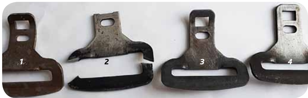
Figure 5. Hardening influence to the mechanical properties. 1 – soft and ductile part without hardening, easily bendable; 2 – hardened part without tempering, really fragile and breaks already applying minor force; 3 – hardened and high temperature tempered, bendable only by applying bigger force; 4 – hardened and tempered with optimum tempering, bendable only slightly and when by applying big force
