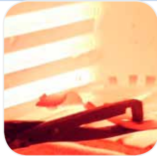
Figure 1. Load removal from a furnace hold in austenizing temperature. Heat treatment temperature can be evaluated by parts glow
